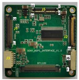
**J1 Interface (HDMI Output):** (Model: USL00-30L-C 30Pin 0.4mm pitch horizontal pin header) Marked with "HDMI\_OUT"
